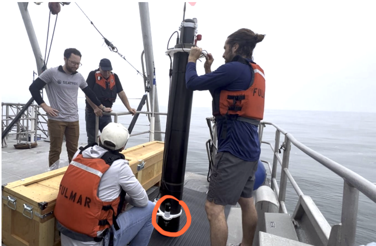
Image 1. PSAP deployment off NOAA's RV Fulmar in Monterey. The icListen hydrophone is circled in red.
