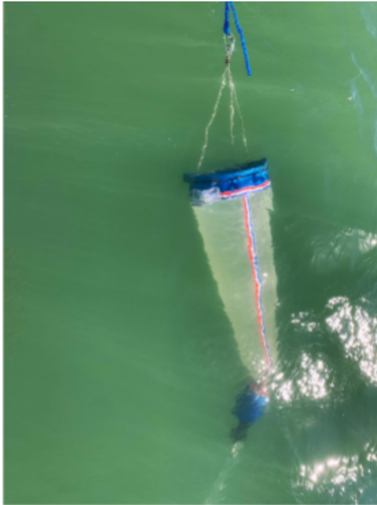
Figure 2. Plankton net intake with hose connector.
