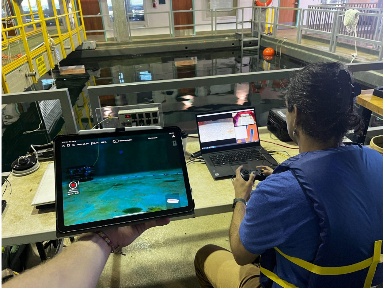
Figure 3: The team during controls testing at the MBARI test tank. The robot, visible on screen, is following a transect line across the bottom of the tank, testing the yaw stabilization and measuring the cycle rate of the planting payload.
