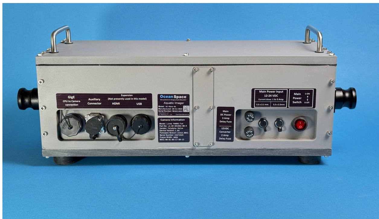
Figure 1. Front (top) and back (bottom) views of the Aquatic Imager imaging unit. Front view shows front- and back-light intensity controls and camera access panel. The back view shows computer and auxiliary connectors, power connections, and on-off switch. 1" ID plumbing connection ports are visible on each side of the imaging unit. Photo: W. Arnold / OceanSpace LLC
