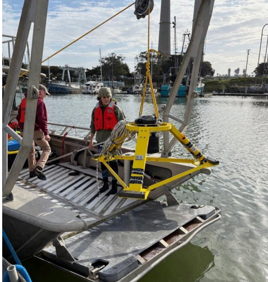
Figure 2. Practice dock-side deployment of the ADCP tripod on the R/V Sheila B. Photo: T.Connolly / MLML
